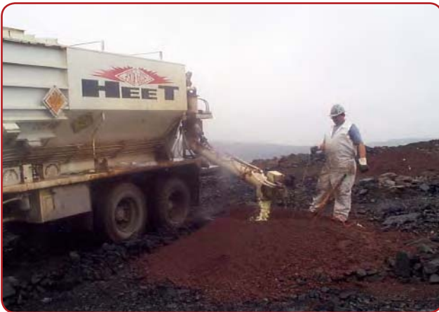
Loading a blast on an iron ore range
