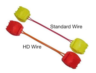
E\*STAR Pronto Connector is an accessory provided for the E\*STAR detonators. It is an assembly of two E\*STAR connectors with an interconnecting wire. It can be used for connection of branches to the firing lines without the need of wire separation, stripping and joining. Simply attach one connector to the branch bus wire and the other to the firing line bus wire and the connection is made. It can also serve as a repair tool to repair a severed or damaged detonator leg wire.
