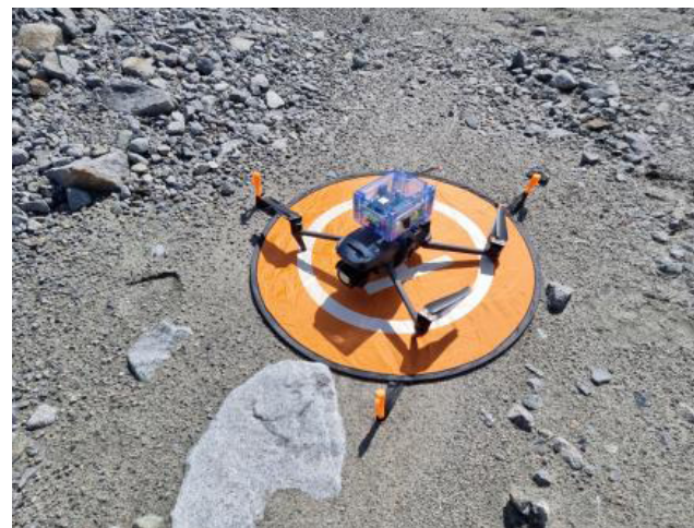
Drone with NOx Sensor Attached
