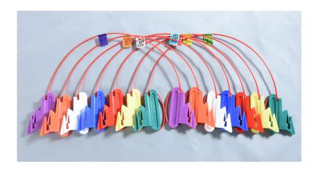
Shock\*Star DC Relay detonators are designed to provide accurate delay timing between the individual rows of blast holes using detonating cord as a primary initiation system. They can be used for developing various delay patterns.
