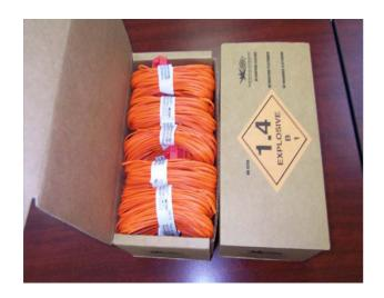
E★STAR Seismic electronic detonators have been designed to provide the precise control necessary to produce the most accurate and consistent seismic record. The E★STAR Seismic detonator may be programmed in 1-millisecond increments from one (1) millisecond up to twenty (20) seconds. using the dedicated DLG 1600-100-S Logger. Unique serial number for each E★STAR Seismic detonator provides "Cradle to Grave" traceability.
