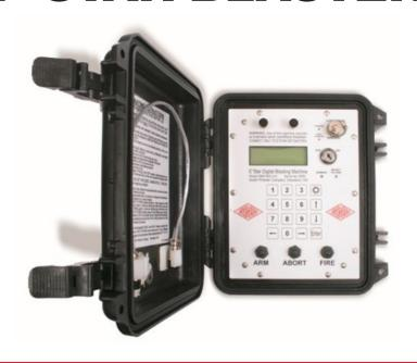
E\*STAR Blaster is a multipurpose device designed to work with E\*STAR detonators. The main functions of the E\*STAR Blaster are to verify charge & fire all detonators in all branches. It is possible to fire up to 1,600 E\*STAR detonators per blast. If connected with second E\*STAR Blaster through E\*STAR Blaster Sync in master-slave mode it is possible to fire up to 3,200 E\*STAR detonators per blast.
