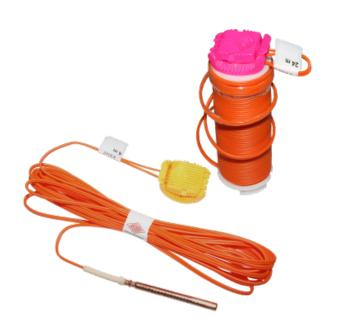
E\*STAR Heavy Duty with its strong wire insulation is robust electronic detonator best suited for harsh blasting conditions. Detonator wires bring higher cut and abrasion resistance which together with special heavy duty Bus-line brings increased leakage protection. E\*STAR HD keeps all the features of standard E\*STAR such as highest safety, timing accuracy and variability of initiation. The E\*STAR HD could be operated with the standard E\*STAR equipment, no special equipment is required.
