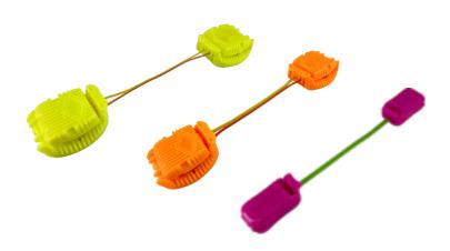
E\*STAR Pronto Connector is an accessory provided for the E\*STAR detonators. It is an assembly of two E\*STAR connectors with an interconnecting wire. It can be used for connection of branches to the firing lines without the need of wire separation, stripping and joining. Simply attach one connector to the branch bus wire and the other to the firing line bus wire and the connection is made. It can also serve as a repair tool to repair a severed or damaged detonator leg wire.
