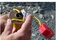
E★Star Detonators contain a capacitor, a logic and timing circuit, and pyrotechnic ignition system manufactured by Special Devices, Inc. This electronic ignition module is integrated with Austin Powder's detonator technology to provide a complete system. When the internal capacitor is charged by the DBM 1600-2KN Digital Blasting Machine, the capacitor provides the necessary energy to initiate the "Ignition Module" and subsequently detonate the Austin Star Detonator 750mg base charge.
