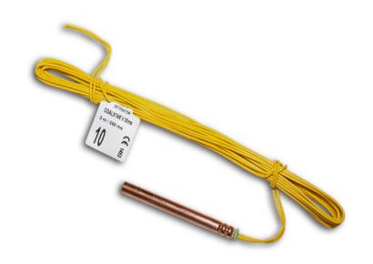
**Coal \*Star 30** are permissible millisecond electric detonators. These detonators are specifically designed for use in environments where there is an ignition hazard associated with air-methane and air-coal dust mixtures. Accuracy of delay times eliminates any overlap and contributes significantly to better breakage and vibration control when properly used. The timing range consists of 17 delay numbers.
