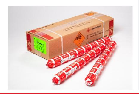
**Emulex 2** is a detonator sensitive emulsion with an excellent combination of velocity of detonation, gas generation characteristics and specific energy. It contains aluminium to enhance heave. Emulex 2 is mainly used for blasting of lumpy broken rock in quarries. Works well as a column load or base charge.
