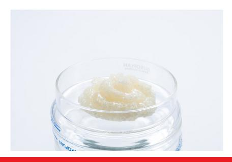
**HEET 30** is a mixture of 30 % of Hydrox S/U and 70 % of ANFO which is produced on site. HEET 30 is augured directly into the borehole by an approved mixing truck.
