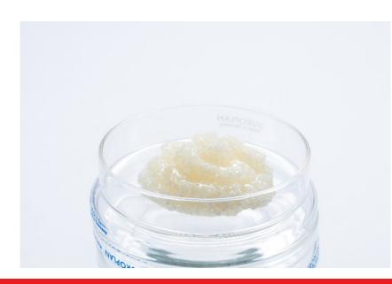
**Hydromite 70** is a booster sensitive bulk emulsion made from a mixture of 70% of Hydrox S/U with 30% low density ammonium nitrate porous prill and fuel oil. This emulsion is sensitized by chemical gassing. Hydromite 70 is widely used in surface mining, quarrying and construction work. As Hydromite 70 is not cap sensitive, it can be initiated by a suitable sized cartridge of Emulex 1 or APB.
