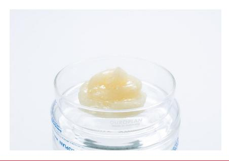
Hydrox U is an emulsion matrix which is used to produce Hydromite 100, Hydromite 70 and HEET 30 by sensitizing with gassing solution(s) in an approved pump truck or repump unit. Hydrox U is a high viscosity matrix and can therefore be also used in up holes.
