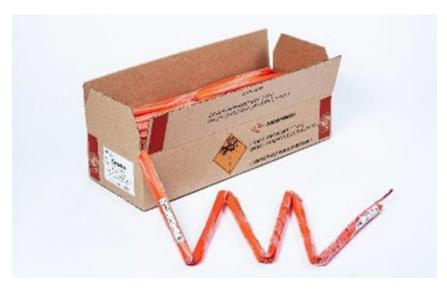
**Emuline** is a cap sensitive emulsion explosive which combines Emulex 1 with detonating cord (12 g/m). It was designed for application in contour boreholes, "pre- splitting" and "postsplitting" applications.
