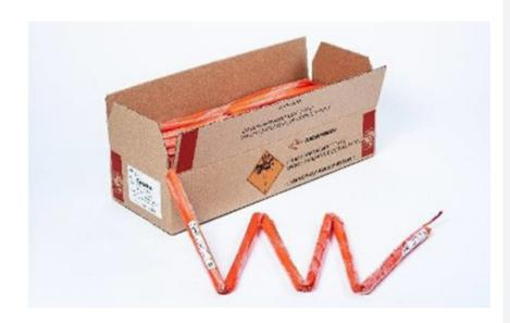
APB-25 consists of a transparent plastic shell (PP), which has a plastic plug (PE) on both ends. The plug on one side has a designated entry point of breakable plastic for easy detonator insertion. The booster charge is made of a plasticized explosive mixture on a PETN basis. APB-25 is mostly used as an underground booster for initiating emulsion explosives (Hydromite 100).
