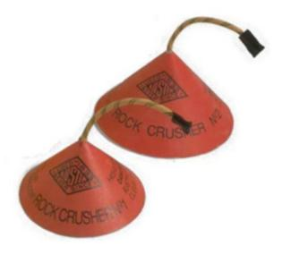
Austin Powder's **Rock Crusher Cast Boosters** are a high-density molecular explosives designed to produce high detonation pressures for optimum initiation of blasting agents. The Rock Crusher family of cast boosters are sensitive to a 450mg PETN base charge detonator or a 25 grain per foot or greater detonating cord.
