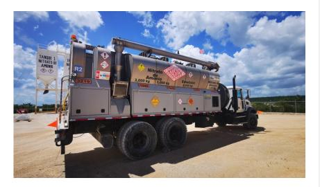
**Hydromite 70** is an emulsion blasting agent, is produced on site from a mixture of 70% of Hydrox S with 30% low density ammonium nitrate porous prill and fuel oil sensitized by chemical gassing.
