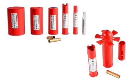
**APB Booster** are initiators for blasting agents and are composed of pentolite (TNT/PETN). APB Boosters are designed to detonate at high velocity and produce a high detonation pressure, ensuring optimal initiation of bulk explosives.
