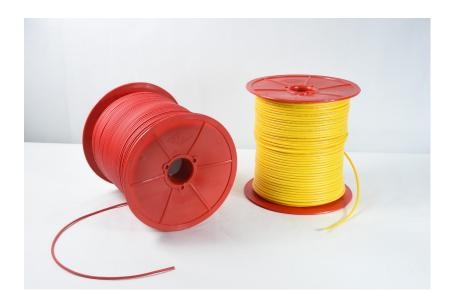
**Detonating Cord** has a core of PETN (pentrite) protected with tapes and multiple polypropylene fibers and is then over-extruded with PVC (Polyvinyl chloride). It is flexible, water resistant and has good tensile strength, enabling reliable use.
