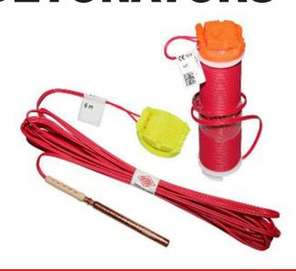
E★STAR electronic detonators feature maximum safety, timing accuracy and initiation selection for most blasting applications. Using the E★STAR Tester equipment it is possible to check the detonators at any time and with the E★STAR Logger equipment it is possible to program them for any delay within the range of 1 to 20,000 ms. With the E★STAR Blaster device it is possible to fire up to 1,600 detonators per blast.
