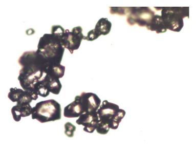
**RDX** is a high explosive used as a raw material in the production of shaped charges, detonating cords, and other components of blasting accessories.
