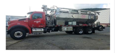
Products in the **HEET Series** are augured blends of ANFO and emulsion for dewatered blast holes in surface operations.
