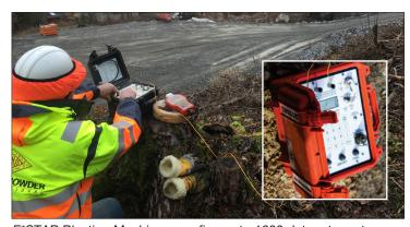
E\*STAR Blasting Machines can fire up to 1600 detonators at one time and can be connected together to fire up to 3200 detonators.
