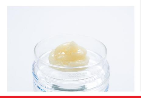
**Hydrox S** is an emulsion matrix which is used to produce Hydromite 100, Hydromite 70 by sensitizing with gassing solution(s) in an approved pump truck or repump unit.
